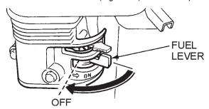
Figure 32. Fuel Valve Lever (Off Position)
